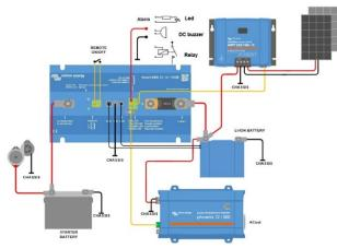
Figure 2: Application example with a MPPT and a Phoenix inverter
